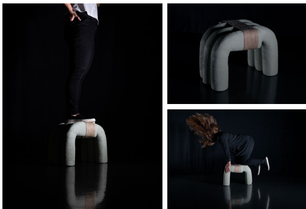
Clasp Stool version 1.0. As object and demonstrating weight-bearing capacity (has supported a minimum of 200 pounds). Mycowelding failed during grow; bound together with hemp cord. Subsequent versions have welded successfully with same or greater weight bearing capacity.
