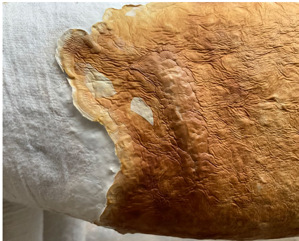
Close-up images to show robust mycelial skin and mycowelding of the Clasp Stool version 3.0. This version is mycowelded together with no additional binders.
